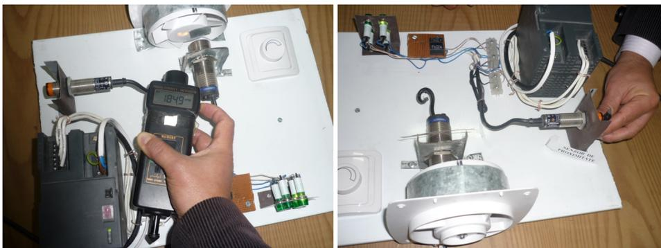
Fig. 6. Determination of the operating parameters of the magnetic sensors
