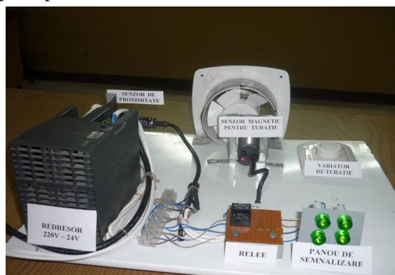
Fig. 5. Electronic assembly used to study the operation of the two types of magnetic sensors
